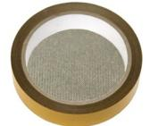
**1** The **glue on EB1 / EB3 is electrically conductive. Therefore the EB1 / EB3 can be stucked under and on the materials. Application under and on nettings, fleeces** to connect the limited width of material. With an adhesive force of 3 N/cm, it sticks relatively poor on difficult under-grounds (e.g. plasterboards). Use a primer first!
